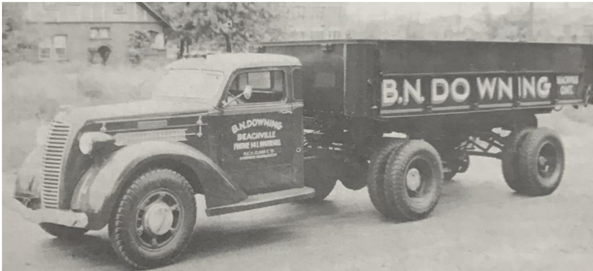
Swank. This isn't the first streamlined Diamond T — it's a '36 — but it conveys the idea - style and lots of it. Note the big hub caps, the vee windshield, the fancy grille and tapered, skirt-sided fenders. And this is only the "standard" version: the "deluxe" job had more of everything.
